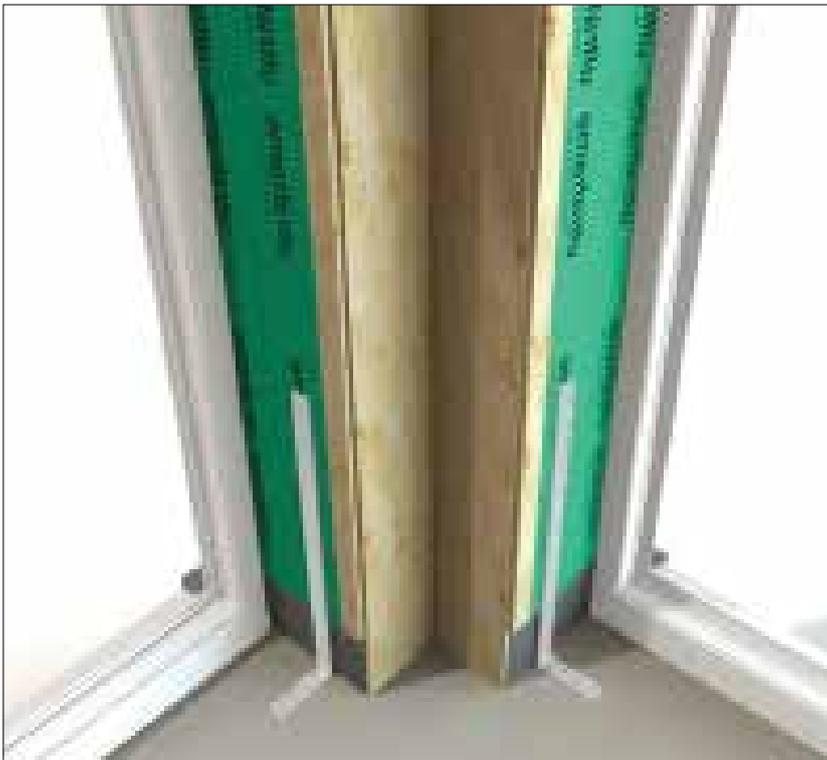
Minimum of 2 straps required. See installation guide for quantity and position of column. For columns on wall, LRP042 (straight support strap) is required running down inside of wall.
