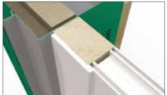
Frame add ons run between columns only and must not run over columns. Where brick plinths are specified, frames require packing with multiple frame add ons or timber and multi-board to space beyond brickwork. It is advisable to use a frame add on for a door next to a column to ensure that hinges do not foul. Check hinge position on door frames.
