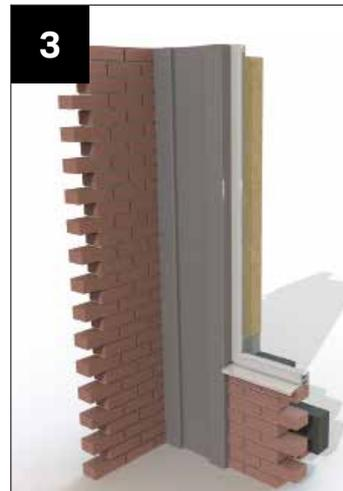
3 Column sat on dwarf wall, claddings
